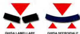
Fig.2 Interazione tra cricca e grafite Interaction between a crack and graphite Interaction entre cricque et graphite
